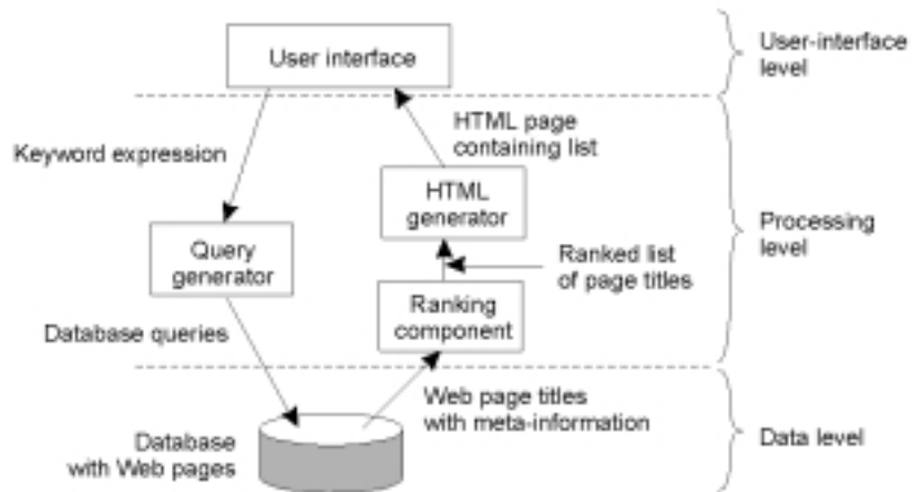
The general organization of an Internet search engine into three different layers
