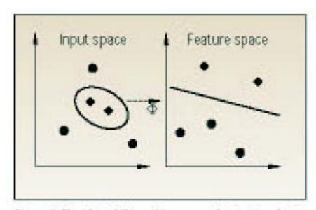
Figure 2. The idea of SV machines: map the training data nonlinearly into a higher-dimensional feature space via  $\Phi$ , and construct a separating hyperplane with maximum margin there. This yields a nonlinear decision boundary in input space. By the use of a kernel function, it is possible to compute the separating hyperplane without explicitly carrying out the map into the feature space.
