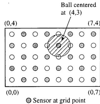
**Figure 1. A checkerboard placement of sensors.**
