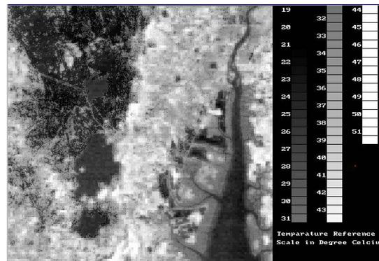
**Figure 3. Kinetic temperature mapping of daytime raw thermal data**
