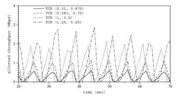
Fig. 14. Allotted throughput with 1 s handoff (one flow).
