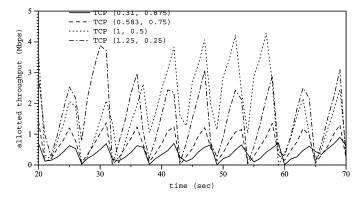
Fig. 13. Allotted throughput with 500 ms handoff (one flow).
