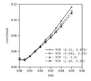
Fig. 12. Overhead over heterogeneous network (100 flows, 100 Mb/s bottleneck, and 10 Mb/s wireless link).
