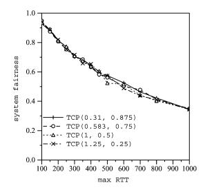
Fig. 17. Fairness with RED gateway (10 Mb/s bottleneck and 20 flows with diverse RTTs).
