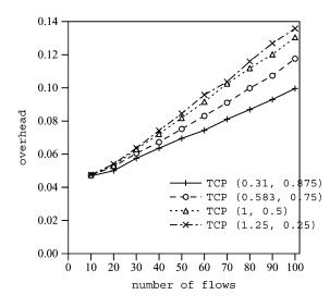
Fig. 4. Overhead over wired network (10 Mb/s bottleneck link).
