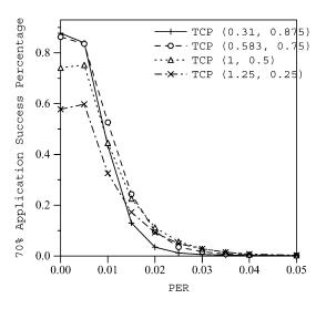
Fig. 15. 70% application success percentage (100 flows, 100 Mb/s bottleneck, and 10 Mb/s wireless link).
