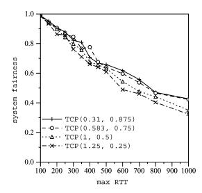
Fig. 16. Fairness with drop-tail gateway (10 Mb/s bottleneck and 20 flows with diverse RFFs).
