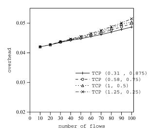
Fig. 5. Overhead over wired network (100 Mb/s bottleneck link).
