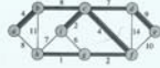
Figure 23.1 A minimum spanning tree for a connected graph. The weights on edges are shown, and the edges in a minimum spanning tree are shaded. The total weight of the tree shown is 37. This minimum spanning tree is not unique; removing the edge (5, 6) and replacing it with the edge (4, 5) yields another spanning tree with weight 37.
