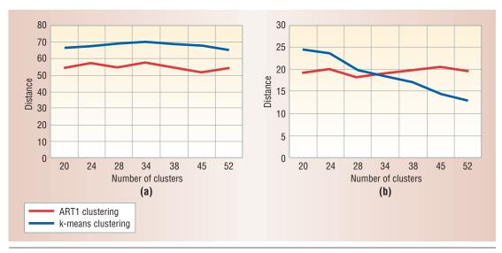
Figure 6. Comparison of ART1 and k-means algorithms. (a) Variations in the average intercluster distance and (b) variations in the average intracluster distance. The ART1 results are quite uniform compared to the k-means algorithm.
