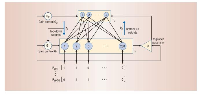
Figure 2. ART1-based clustering architecture. The pattern vector  $P_{H}$ , which represents the access patterns of the host H, is the input to the comparison layer  $F_1$ . The vigilance parameter  $\rho$  determines the degree of mismatch to be tolerated. The nodes at the recognition layer  $F_2$  represent the clusters formed. Once the network stabilizes, the top-down weights corresponding to each node in  $F_2$  represent the prototype vector for that node.
