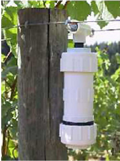
Fig. 4 – A sensor node deployed in vineyard. http://www.intel.com/technology/techresearch/research/rs01031.htm .
