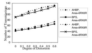
Fig. 15. Performance comparison of BPS and AHBP under nonuniform propagation. Network density = 6.25.
