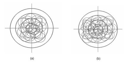
Fig. 6. (a) Example of a distorted figure for a 4R X 4R region with 64 nodes. The number of transmissions is 21. (b) Example of a distorted figure for a 6R X 4R region with 96 nodes. The number of transmissions is 32.
