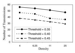
Fig. 4. Effect of Th on the performance of BSP. Network size = 6R X 6R.
