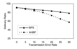
Fig. 13. Performance comparison of BPS and AHBP in the presence of transmission errors. Network size =  $6T \times R$ . Number of nodes = 144.
