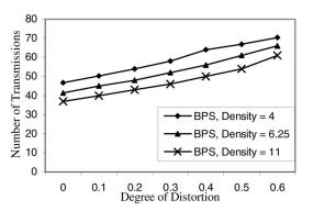
Fig. 14. Effect of nonuniform propagation on BPS. Network size is 1,800 m X 1,800 m.
