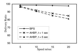
Fig. 12. Effect of mobility on different protocols. Network size is  $8R \times 8R$ . Number of nodes = 144.
