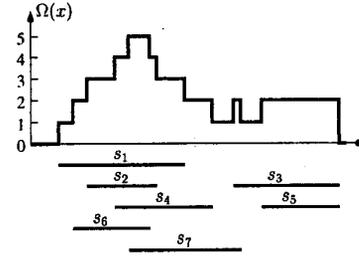
Figure 3: The overlap function for a set of 7 sensors.
