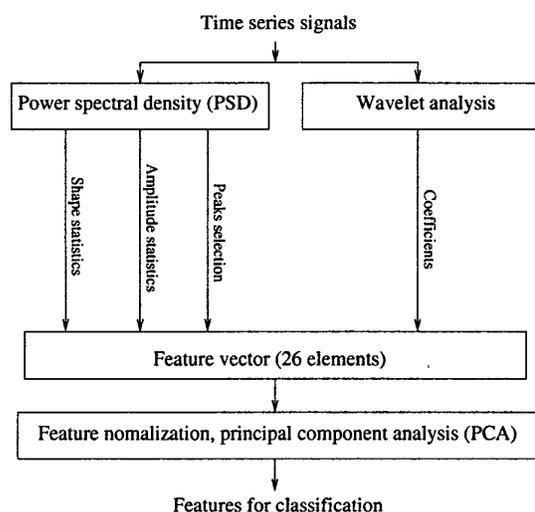
Figure 1: Block diagram of the feature extraction procedure.
