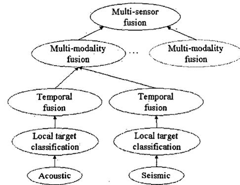
Figure 2: The hierarchical structure of three levels of data fusion.
