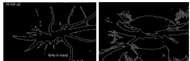
Fig. 2: Original Image Contour Extractions Using Canny Edge Detector (Because the Fundus image's B/W image is originally converted from a color image, the vessels are not as clear as those of IVFA images'.)
