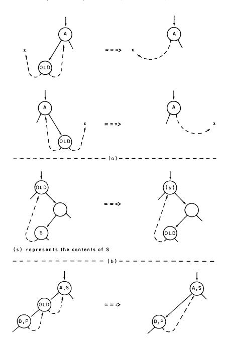
Figure 7. Deletion of a node by (a) direct removal; (b) replacement; (c) circumvention
