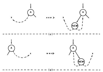
Figure 5. Insertion of a new node when (a) KEY(NEW) < KEY(A); (b) KEY(NEW) > KEY(A)
