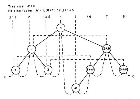
Figure 3. A balanced and threaded tree structure with even total number of nodes
