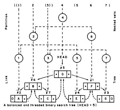
Figure 2. Process of balancing and threading a tree with odd total number of nodes
