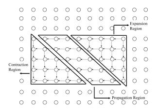
Fig. 5. Expansion, Propagation and Contraction Regions in an  $\Xi_3$  Contour.
