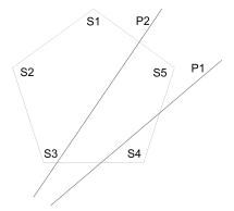
Fig. 3. A cluster formed with five sensors.
