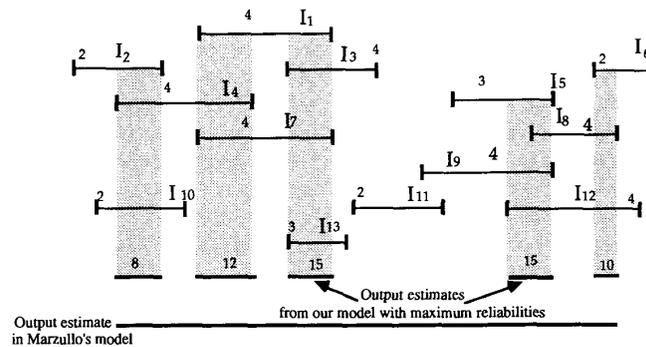
Fig. 3. A comparison of output estimates from Marzullo's method of integration and our method. The shaded strip illustrates overlapping regions of three or more interval intersections, where  $n = 13$ ,  $f = 10$ , and  $n - f = 3$ .
