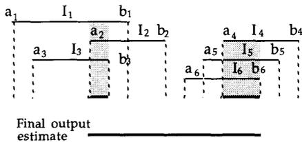
Fig. 1. Integrated interval estimates (*a la* Marzullo) ( $a_1 < a_3 < a_2 < b_3 < b_1 < b_2 < a_6 < a_5 < a_4 < b_6 < b_5 < b_4$ ).
