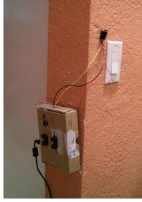
Fig. 2. Placement of a node at a crossing. The light sensor is placed outside, pointing towards the light source of a region.
