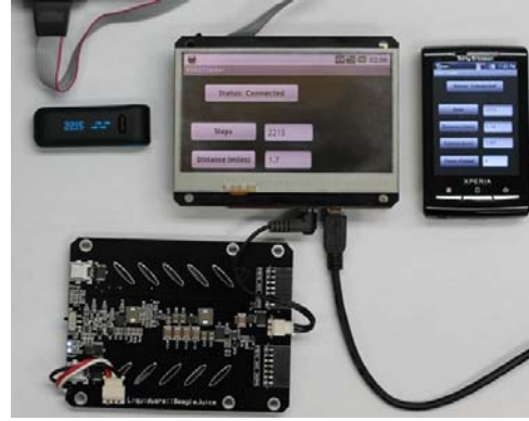
Fig. 9. Snapshot of testbed for FitLock, consisting of BeagleBoard and Xperia devices used as Fitbit trackers.
