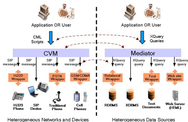
**Figure 1: Analogy between CVM and Data Mediator.**
