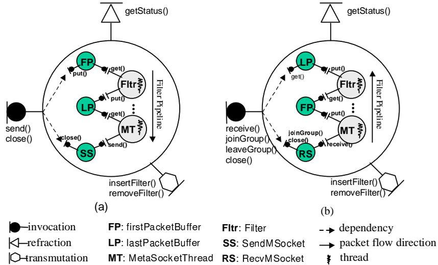
Fig. 2. MetaSocket architecture: (a) MetaSendMSocket; (b) MetaRecvMSocket.
