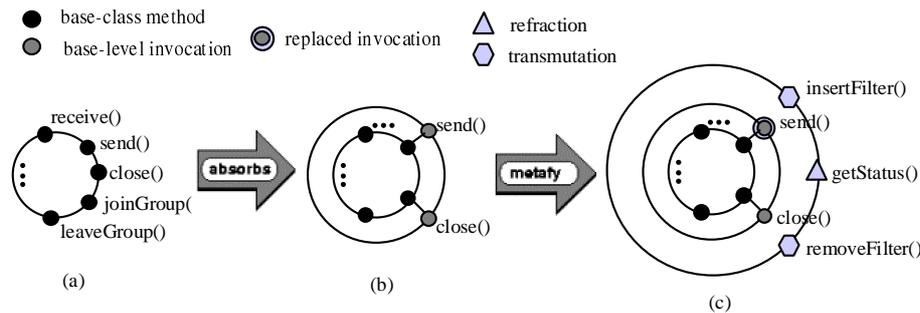
**Fig. 1.** MetaSocket absorption and metafication. (a) Java MulticastSocket; (b) SendMSocket component; (c) MetaSendMSocket meta-level component.
