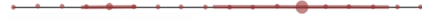
Figure 4: Viewing histograms along edges are computed by dividing the edge in segments and monitoring gaze-count in each segment.
