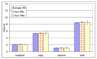
Figure 9: The per-VM migration time when different numbers of VMs, each with a 512MB memory, were migrated in sequence. A RAMFS on the destination host was used to store the migrated VM states.
