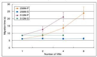
Figure 16: The comparison of per-VM migration time for four VMs between parallel and sequential migration.
