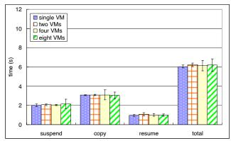
Figure 7: The per-VM migration time when different numbers of VMs, each with a 256MB memory, were migrated in sequence. A RAMFS on the destination host was used to store the migrated VM states.
