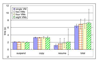
Figure 6: The per-VM migration time when different numbers of VMs, each with a 256MB memory, were migrated in sequence. A local disk on the destination host is used to store the migrated VM states.
