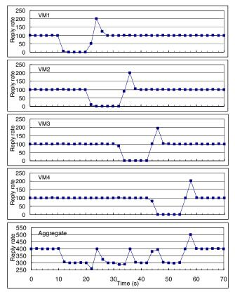
Figure 14: The throughput of web servers running on four VMs that were under migration.
